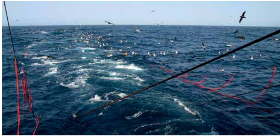
Twin bird-scaring lines keep birds away from the danger zone behind a Namibian trawler
